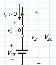
**Problem:** The voltage across a zener diode in breakdown is NOT EXACTLY equal to  $V_{ZK}$  for all  $i_z > 0$ . The CVD is an approximation.
