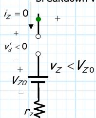
Analyzing this Zener PWL model, we find that **if** the model voltage  $v_Z$  is less than  $V_{ZO}$  (i.e.,  $v_Z < V_{ZO}$ ), then the **ideal** diode will be in **reverse** bias, and the model current  $i_Z$  will equal zero. In other words:
