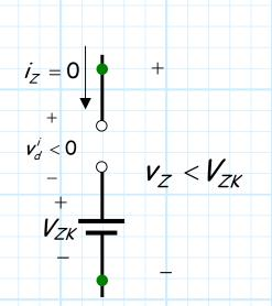
Analyzing this Zener CVD model, we find that **if** the model voltage  $v_Z$  is less than  $V_{ZK}$  (i.e.,  $v_Z < V_{ZK}$ ), then the **ideal** diode will be in **reverse** bias, and thus the model current  $i_Z$  will equal **zero**. In other words:
