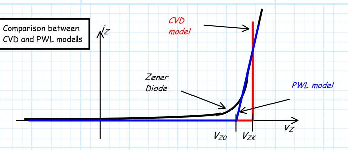
Q: How do we construct this PWL model (i.e., find  $V_{70}$  and  $r_{7}$ )?
