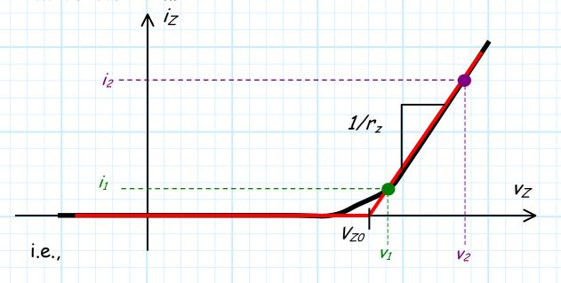
$$r_z = \frac{V_2 - V_1}{i_2 - i_1}$$
